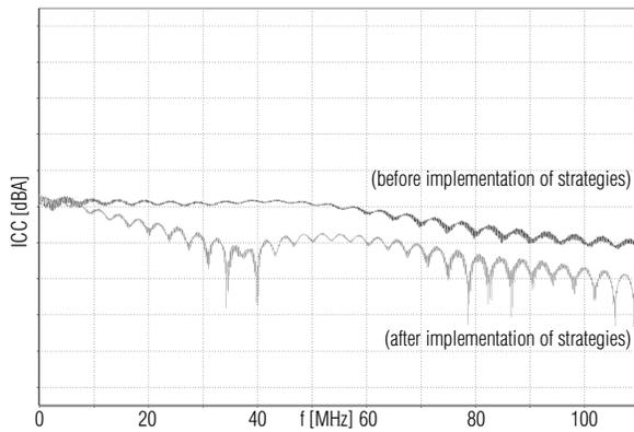
**Fig. 1** Power supply current of drive circuit
