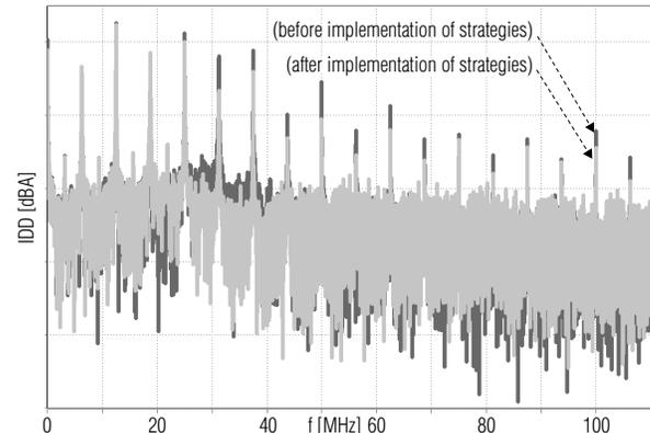
**Fig. 2** Power supply current of digital circuit
