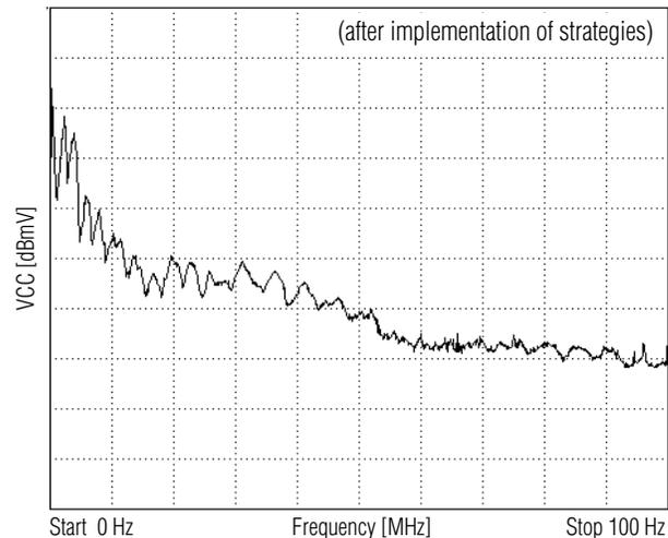
**Fig. 3** Results of spectrum measurements for power supply voltage on driver
